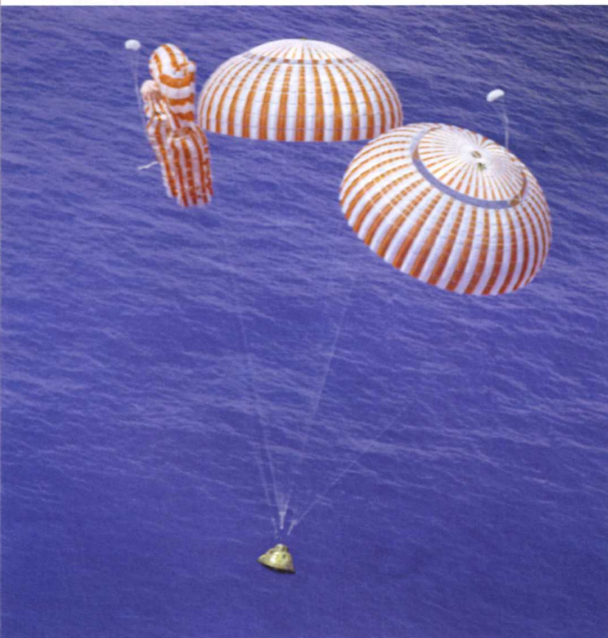
BELOW The Apollo 15 Command Module 'Endeavour', with Astronauts David R. Scott, Alfred M. Worden and James B. Irwin aboard, nears a safe touchdown in the mid-Pacific Ocean to end their lunar landing mission. Although causing no harm to the crewmen, one of the three main parachutes failed to function properly. The splashdown occurred at 3:45:53pm on 7th August 1971, some 330 miles north of Honolulu, Hawaii. (NASA)
