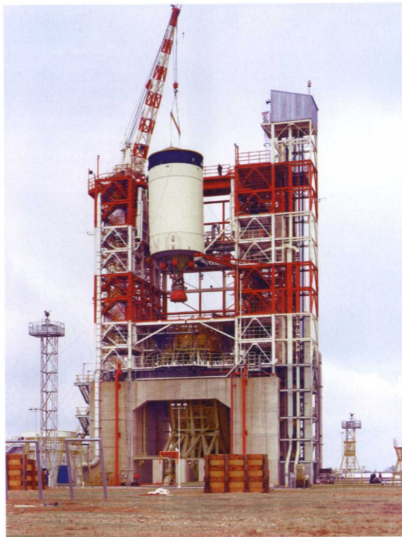
ABOVE An S-IVB, Saturn V final stage is winched onto its test stand. (NASA)
