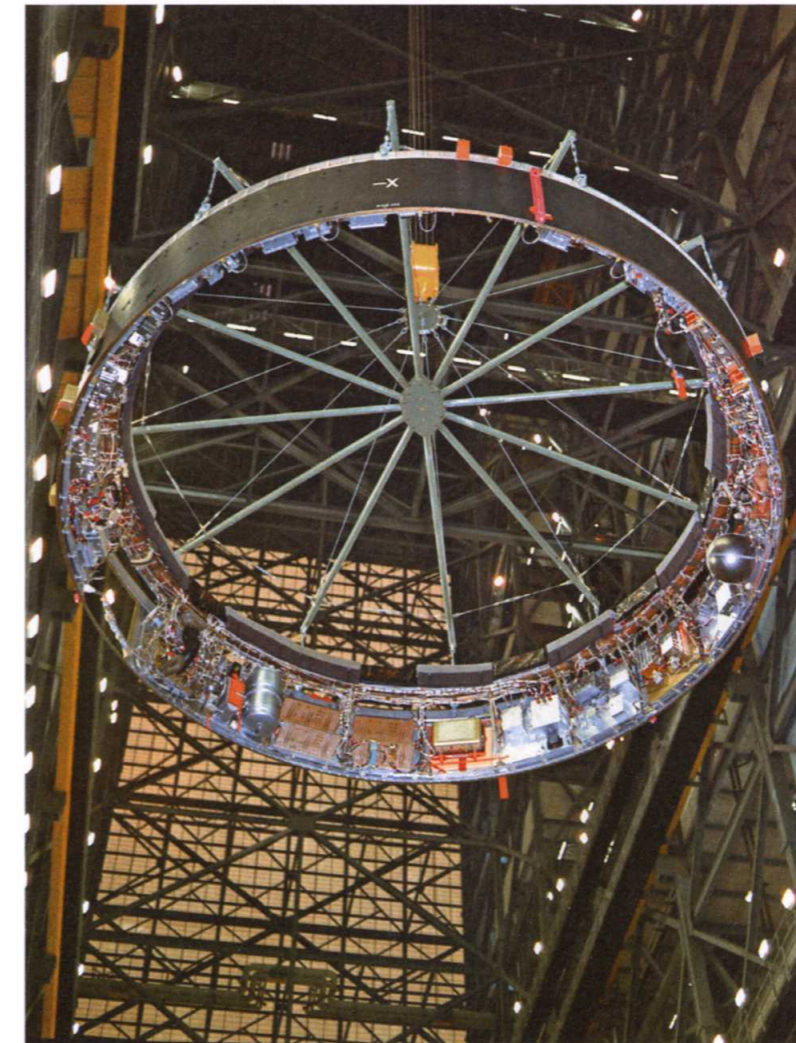
ABOVE This photograph was taken during the final assembly operation of the Saturn V launch vehicle for the Apollo 4 (SA-501) mission. The Instrumentation Unit (IU) is being hoisted to be mated to the S-IC/S-II assembly in the Vehicle Assembly Building high bay at the Kennedy Space Center. (NASA)
