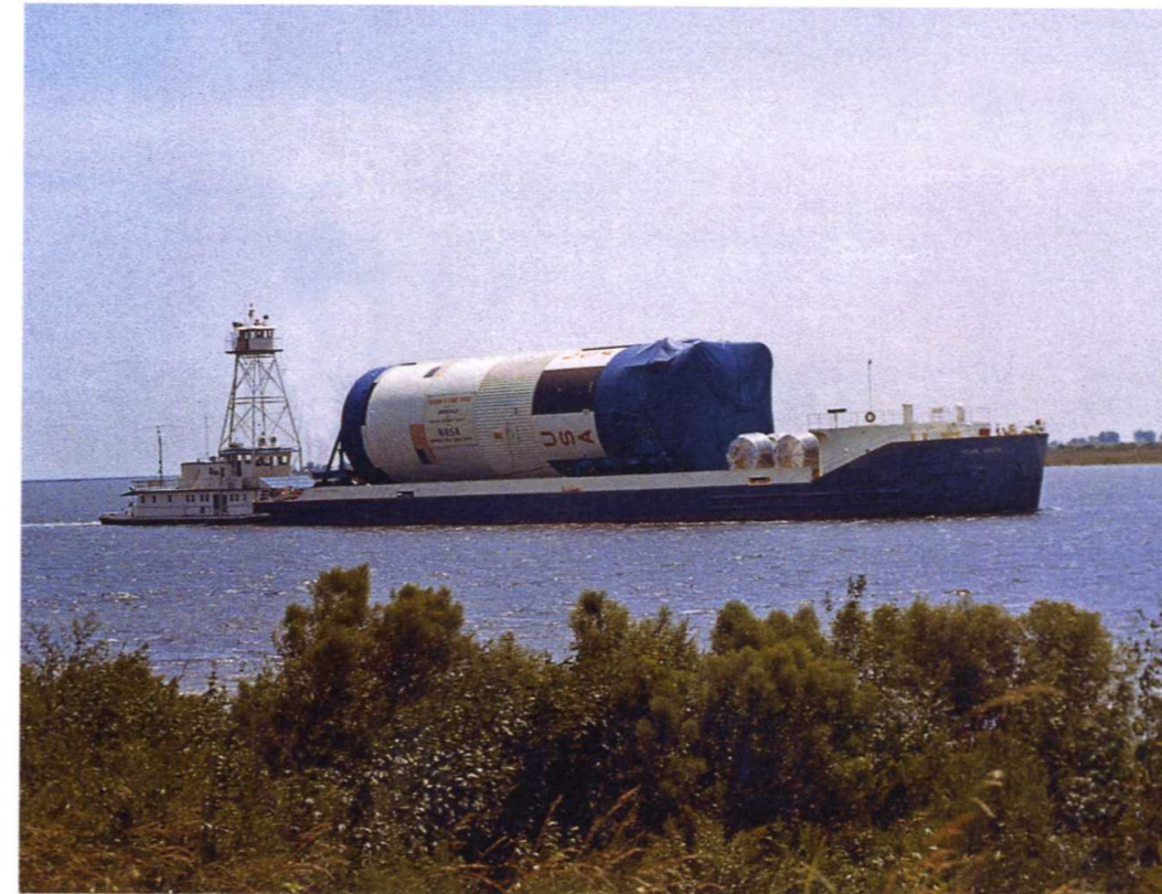
LEFT A Saturn V S-1C first stage aboard NASA barge Pearl River returning from the Mississippi Test Facility to the Michoud Assembly Facility. (NASA)
