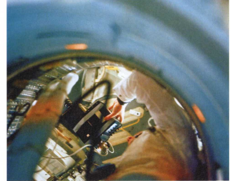
ABOVE Neil Armstrong floats in the tunnel connecting the LM and CM, using the Westinghouse color TV camera to document Buzz doing a LM inspection. An extra TV monitor is attached to the camera with tape to aid filming. (NASA)
