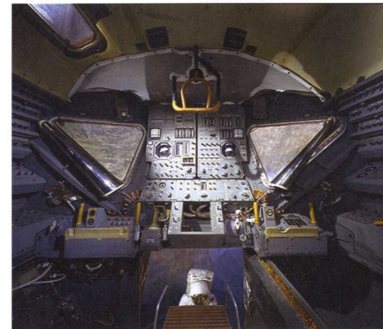
BELOW A view inside the Lunar Module ascent stage looking forward towards the windows and main control panels. (Smithsonian Institution Negative No.SI-2001-2947-A)
