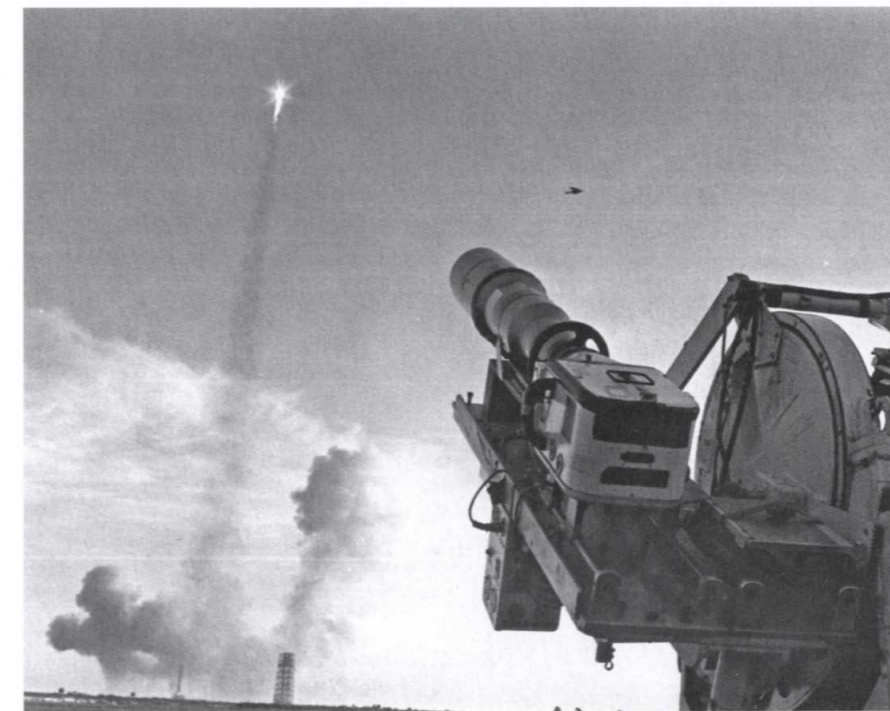
ABOVE A telescopic ground tracking camera at KSC follows the flight path of Apollo 8. (NASA)
