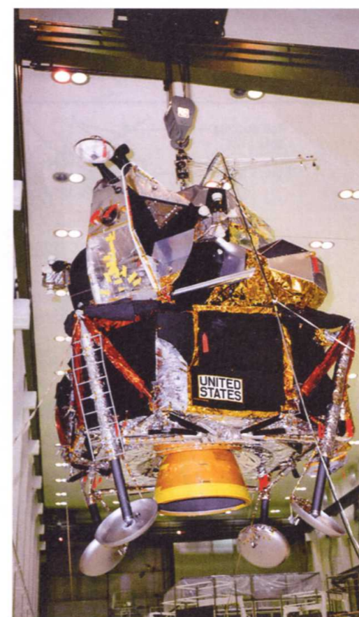
material that crushed on contact with the lunar surface, to help absorb the impact. There was no need for the legs to rebound with a complex hydraulic mechanism, as each LM was only ever going to make one landing. At the end of each leg was a giant footpad designed to land
