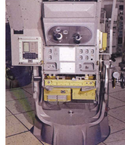
LEFT A ground-based mock-up of the Apollo GNCS in the MIT lab. The unit carries the sextant and wide-field telescope optics, the computer processor racks (gold) and the control panel and DSKY needed to link it all together. (The Charles Stark Draper Laboratory, Inc)
