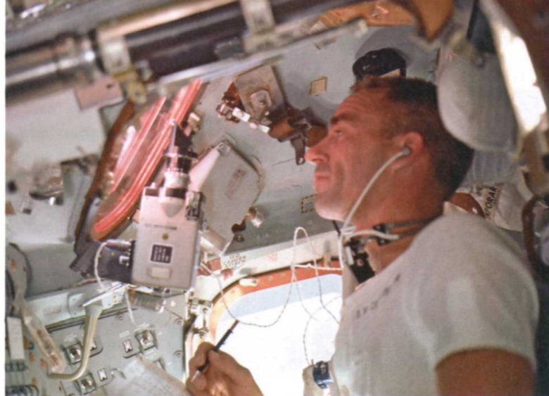
ABOVE Walt Cunningham gets to grips with the sextant star sighting system on board Apollo 7 – the CM's maiden flight in Earth orbit. (NASA)
