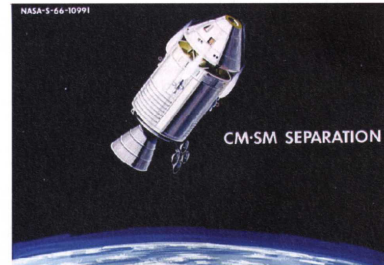
ABOVE Artist's impression of the moment of jettison of the Service Module from the Command Module – prior to re-entry. (NASA)
