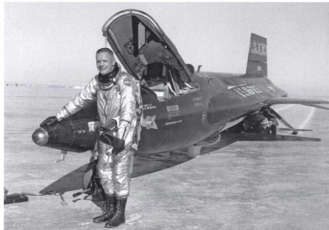
RIGHT Dryden pilot Neil Armstrong is seen here next to the first X-15 after a research flight. The X-15 was a rocket-powered aircraft, 50ft long with a wingspan of 22ft. (NASA)
