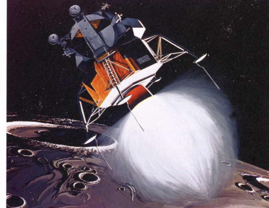
material that crushed on contact with the lunar surface, to help absorb the impact. There was no need for the legs to rebound with a complex hydraulic mechanism, as each LM was only ever going to make one landing. At the end of each leg was a giant footpad designed to land
