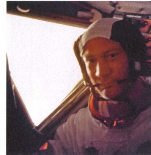
LEFT The snoopy cap housing headphones and a microphone – worn here by Buzz Aldrin inside the 'Eagle' lander on the surface of the Moon. (NASA)
