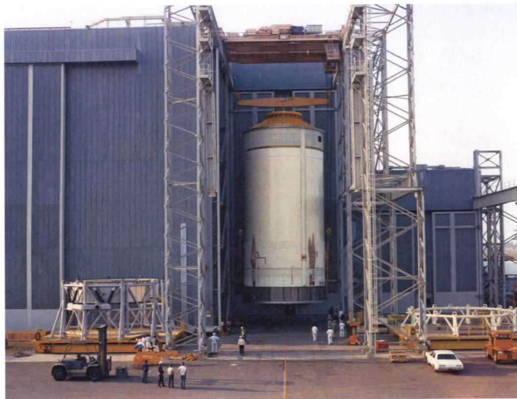
BELOW The Saturn V S-II (second) stage for the Apollo 6 mission being lowered atop the S-IC (first) stage during the final assembly operations in the Vehicle Assembly Building (VAB) at the Kennedy Space Center. (NASA)
