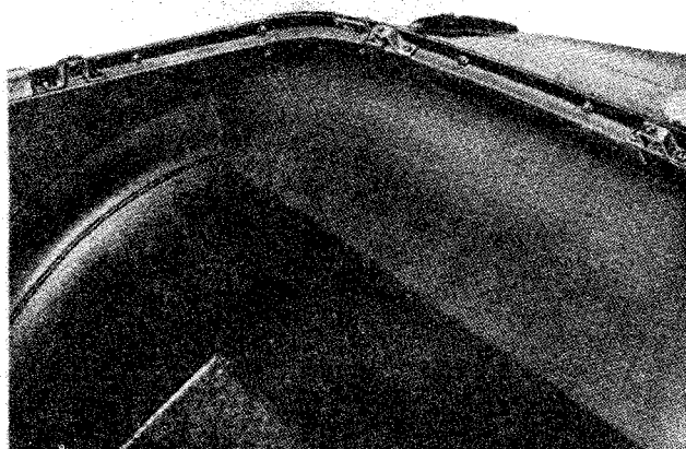
Fig. 5 Bridge Pieces in position on Elbow Rail Channel.
