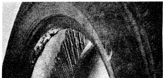
Fig. 4 Running deflated destroyed this Tyre.
