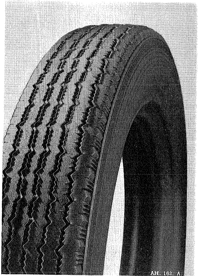
Fig. O.18. Fins or feathers caused by severe misalignment. With minor misalignment, probably aggravated by road camber, the ribs may have sharp edges instead of upstanding fins. These conditions will usually be accompanied by heel and toe wear across the tread due to its being distorted and worn away laterally instead of in a true rolling direction.
