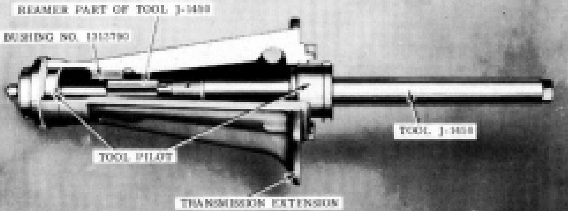
Fig. 353. Installing Transmission Extension Bushing
