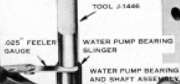
Fig. 212. Installation of Water Pump Shaft Slinger
