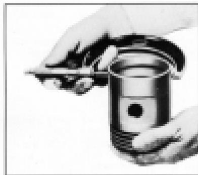
Fig. 185. Measuring Piston
