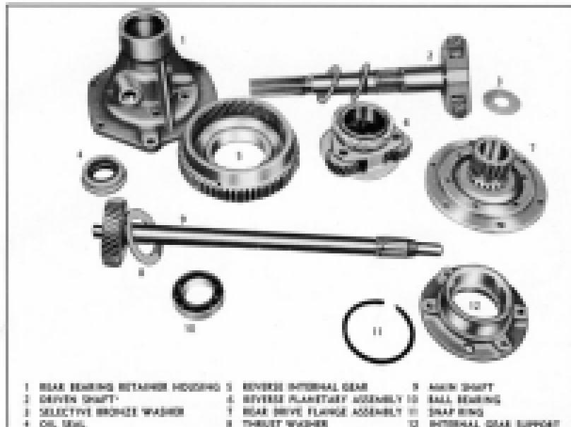
Fig. 441. Disassembled View of Rear Assembly.
