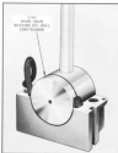
Fig. 185. Installing Rear Main Bearing Oil Seal in Main Bearing Cap
