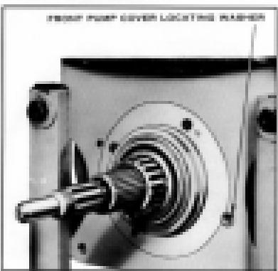
Fig. 495. Installing Pump Cover Locating Washer
