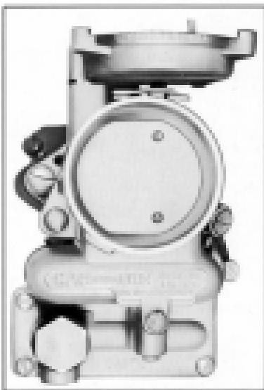
Fig. 213. Automatic Choke Valve.
