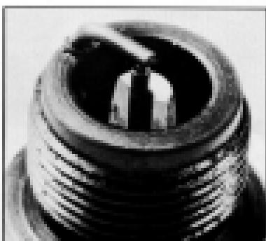
Fig. 608. Spark Plug Insulator Broken at Lower End
