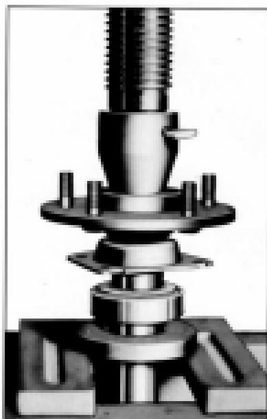
Fig. 129. Installing axle shaft bearing with tool J-647
