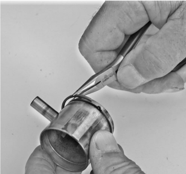
FIG. 6-10. Long-nosed pliers also help, but be careful not to twist the rings or stretch them open more than necessary. Robert Shelby
