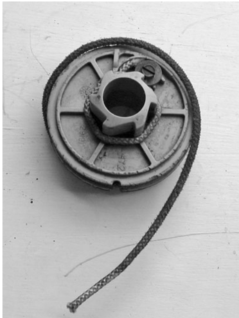
FIG. 5-10. A toothed wheel transmits starter torque to the crankshaft. Robert Shelby
