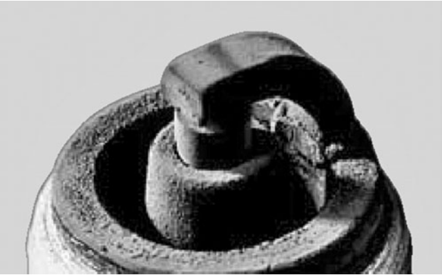
FIG. 2-10. The darker the color of the insulator, the richer the mixture. U.S. Bosch
