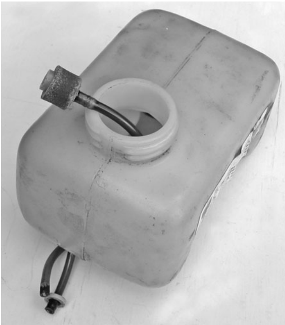
FIG. 2-3 In-tank filters should be changed annually and whenever the equipment comes into the shop. Robert Shelby
