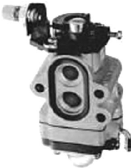
FIG. 1-16. The Walbro WYA carburetor features a 12-mm bore, an adjustable idle jet, and can be fitted with an accelerator pump. While designed for stratified-charge two-stroke engines, this carburetor can also be adapted to four-strokes.
