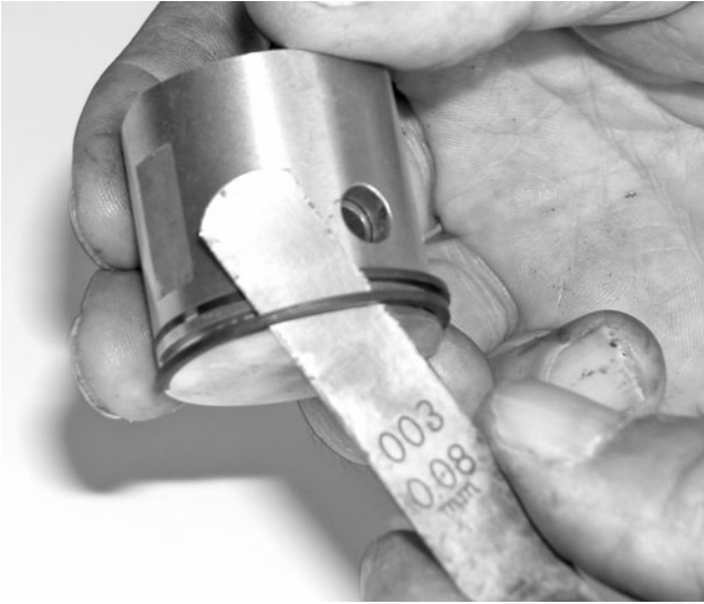
FIG. 6-9. A feeler gauge can be used like a tire tool to pry rings out of their grooves. When installing the lower ring, the gauge acts as a bridge over the upper groove. Robert Shelby
