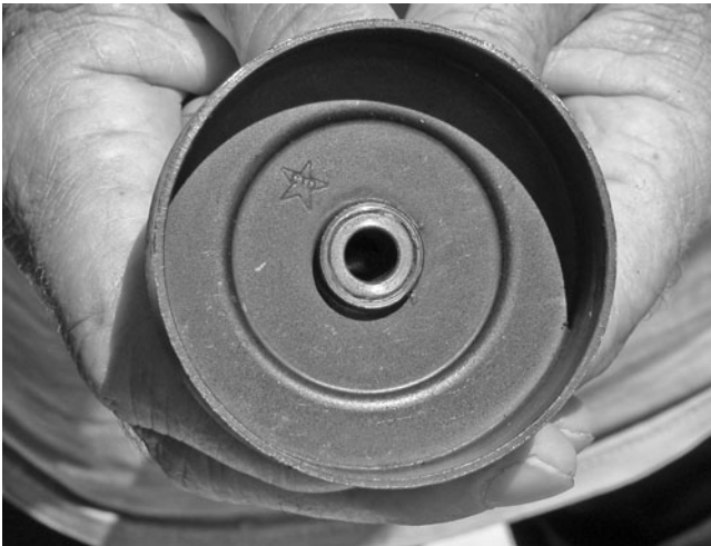
FIG. 7-2. When the clutch drum rides on a bushing, frequent lubrication is required. Robert Shelby
