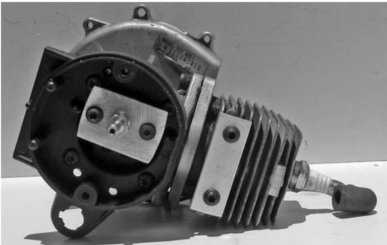
FIG. 6-2. The crankcase and cylinder for this engine share the same casting, which means that both the intake and exhaust ports must be sealed. Robert Shelby
