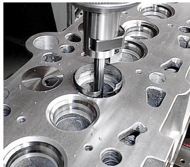
Picture 4 - Removing the thin wall of the old valve seat insert
