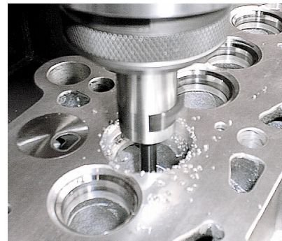
Picture 5 - Cutting the counter bore
