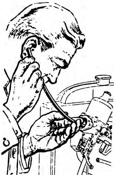
Fig. 16: Synchronization may be tested using rubber tube as stethoscope, but Uni-Syn is more accurate.
