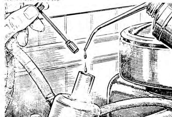
Fig. 8: Adding Oil to the carburettor dashpots.
