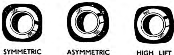
Fig. 4: The three types of distributor cam, as seen from above. Point gap and dwell angle specifications for each type are given in the text.
