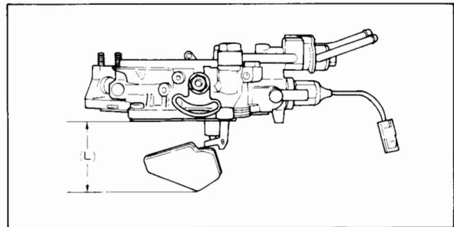
45. Install air horn on main body with two (longest) screws near fuel inlet.
