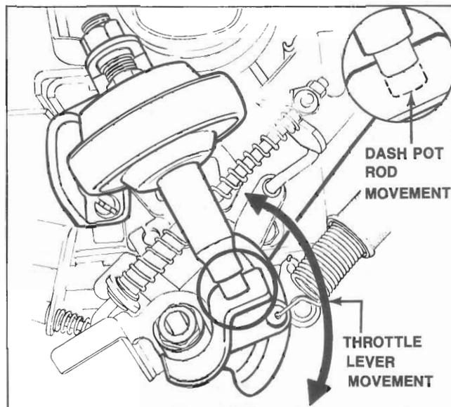
5. Start the engine and warm up the engine to the normal operating temperature. Make sure the engine operates at the specified idle speed. Operate the throttle lever until it is away from the dash pot rod.
