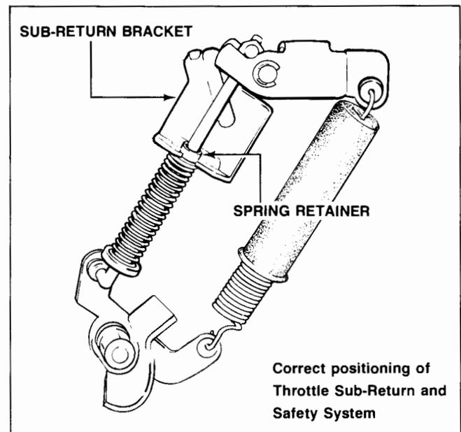
50. Complete installation of the sub-return bracket by installing side screw into main body.
