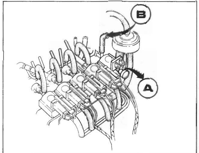
3. Disconnect the coupler from the solenoid valve and connect battery power to the terminal on the valve.
