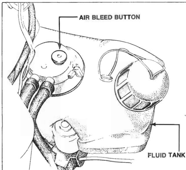
4. Turn the ignition key to the "START" position and make sure that the starting assist fluid does not spout from the nozzle of the carburetor. [Ambient temperature should be **above -18°C (0°F)**]
