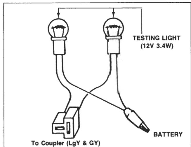
6. If the current does not start to flow to both terminals simultaneously, remove the cap from the throttle sensor adjusting screw.
