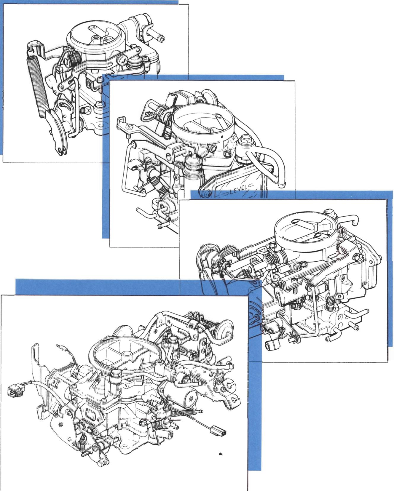
Originally the carburetor was called a mixing valve which, as the name implies, is basically what it did; it mixed air and fuel into a highly combustible state.
