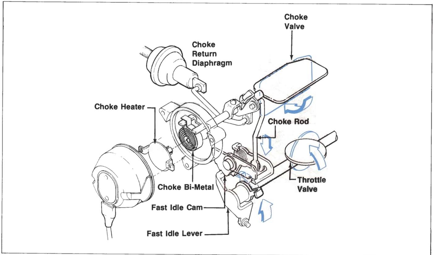
While the choke is on, a fast-idle system is also used to help prevent stalling and to provide a smooth idle. The fast-idle is operated by the choke linkage and is used to increase idle speed.
