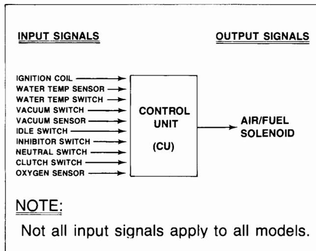
To help you diagnose the **Closed Loop System** and make sure the CU is receiving all the necessary signals, Mazda has introduced the **System Checker '83** as a diagnostic aid.
