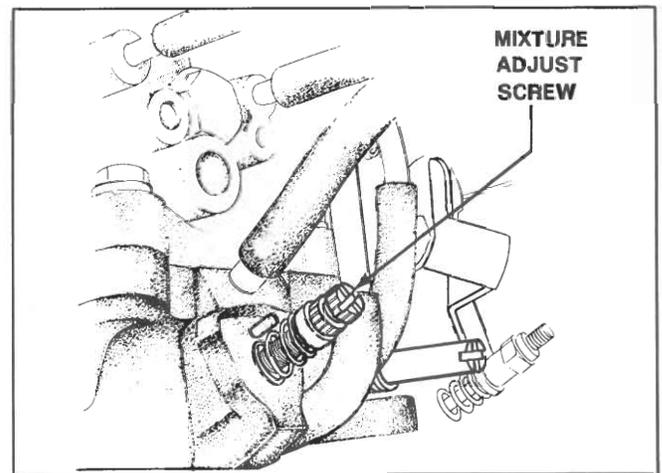
4. Set the idle speed at the highest rpm by turning the mixture adjust screw.
