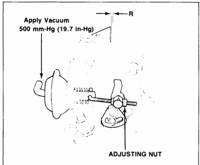
5. Measure the temperature around the bi-metal and compare the clearance (**R**) with the specifications.
