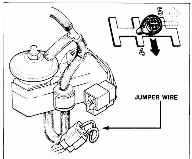
11. Slowly increase the engine speed from idle and check the engine speed at which current begins flowing. The difference between the engine speeds recorded in Steps 10 and 11 should be  $150 \pm 70$  rpm.
