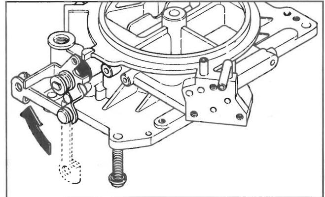
46. Connect fast idle rod by using cotter pin.
