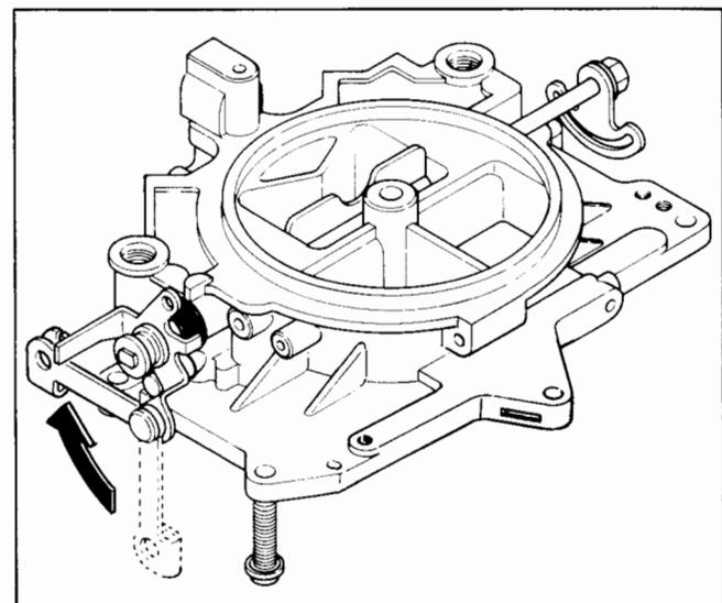
49. Install the bi-metal spring housing as follows:
