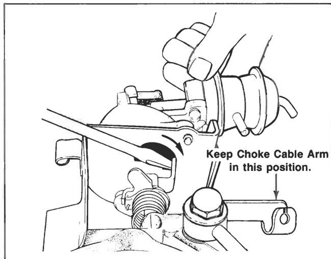
If necessary, use a screwdriver to assist in aligning the choke shaft lever and the bi-metal spring, but be careful not to damage the bi-metal or heater element by doing so.
