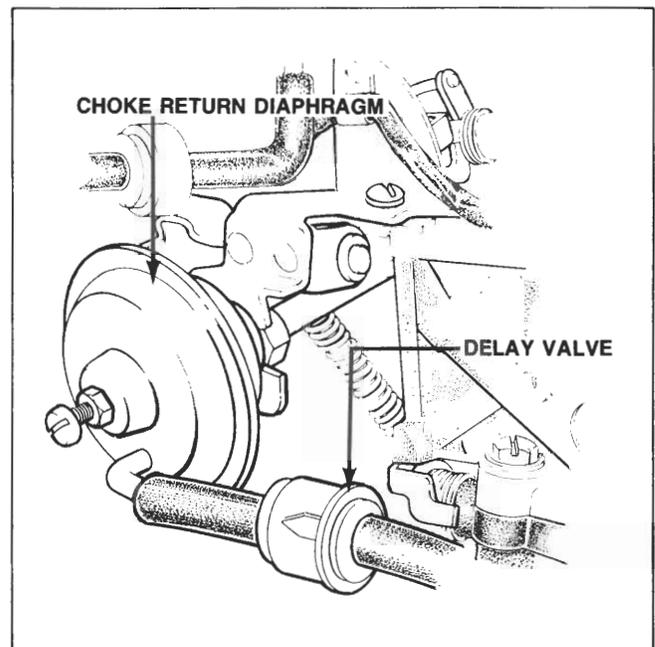
● **CHECKING CHOKE RETURN SOLENOID VALVE (Except for California & Canada- 1980)**
