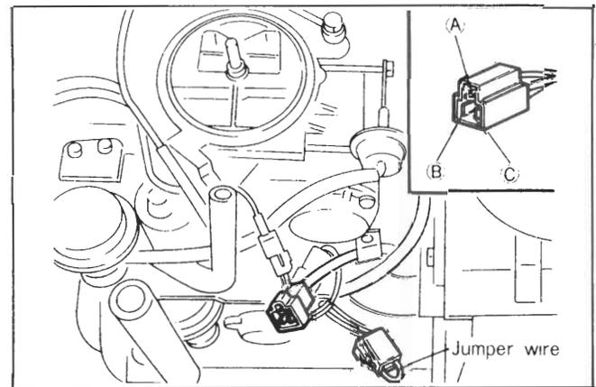
4. Connect a voltmeter to the main air bleed control solenoid (Br) terminal and ground.
