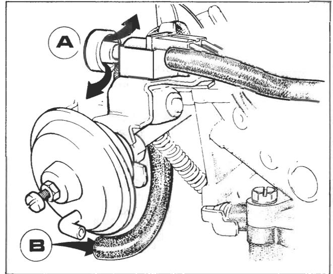
3. Disconnect the coupler from the solenoid valve and connect battery power to the terminal on the valve.
