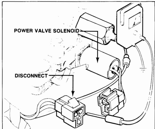
• **Signal Inspection (Automatic Transmission- Except for California)**
