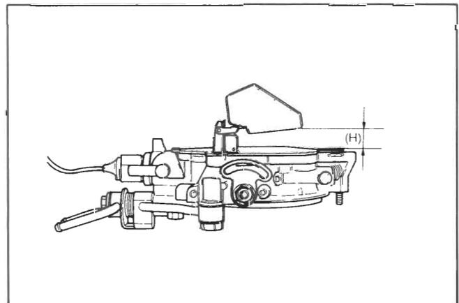
This clearance should be  $16 \pm 0.5 \text{ mm}$  ( $0.63 \pm 0.02 \text{ in}$ ). If the clearance is not within specifications, bend the float seat lip until the proper clearance is obtained.
