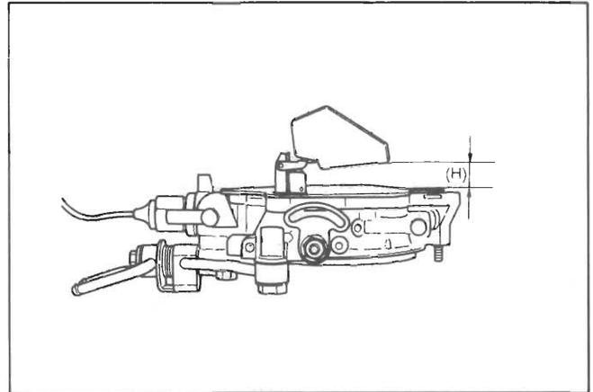
Turn the air horn to the normal position and allow the float to lower by its own weight. Measure the distance (**L**) between the bottom of float and the air horn gasket. The clearance should be  $51 \pm 0.5$  mm ( $2.0 \pm 0.02$  in). If the clearance is not within specifications, bend the float stopper until the proper distance is obtained.
