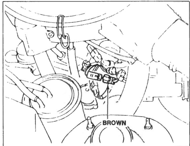
4. Connect the negative probe of the voltmeter to each terminal (**GY and LgY**) and connect the positive probe to the **B** terminal of the alternator.
