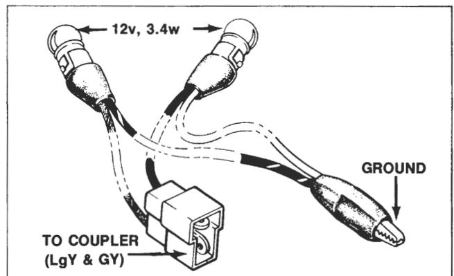
6. If the current does not start to flow to both terminals simultaneously, remove the cap from the throttle sensor adjusting screw.
