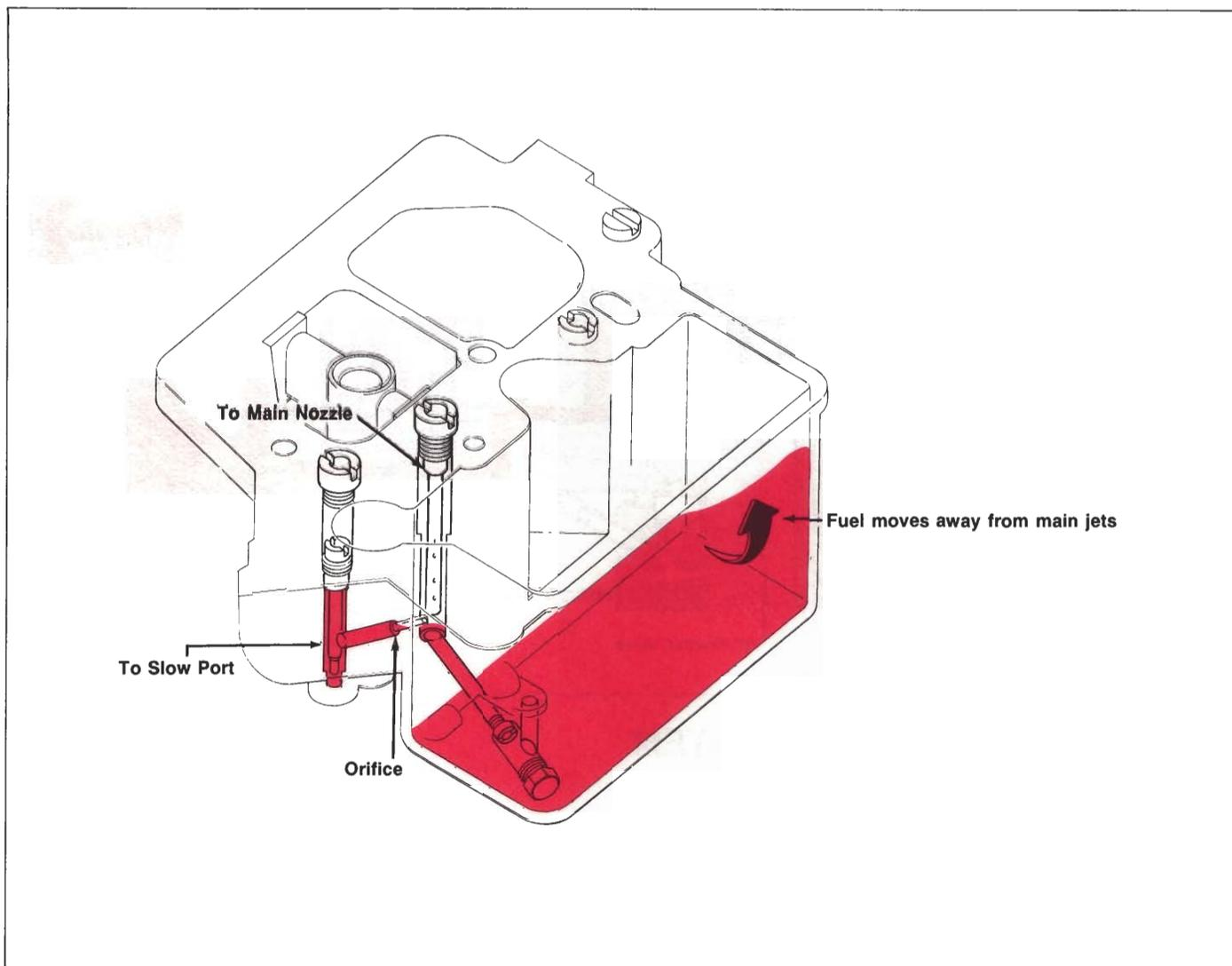
Due to the location of the carburetor on the FWD GLC, during fast left hand turns centrifugal force will cause the fuel to flow as shown.
