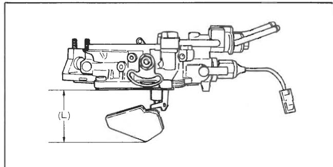
40. Install air horn on main body with two (longest) screws near fuel inlet.\*
