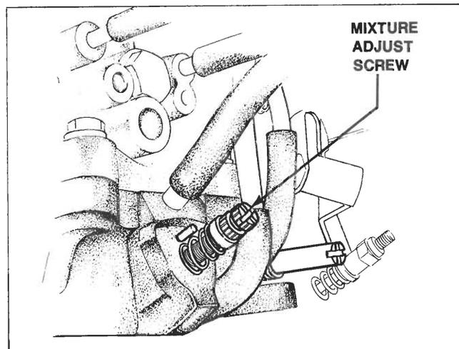
4. Set the idle speed at the highest rpm by turning the mixture adjust screw.
