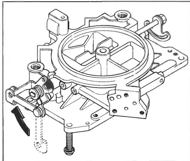
41. Connect fast idle rod by using cotter pin.
