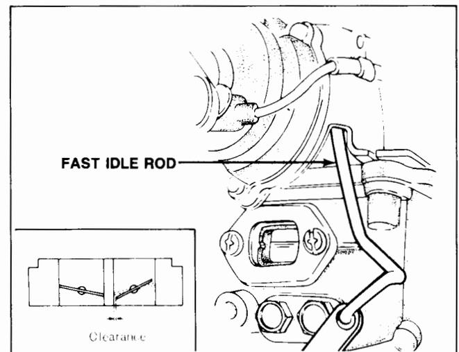
If the clearance is not within specifications, bend the fast idle rod until the proper clearance is obtained.
