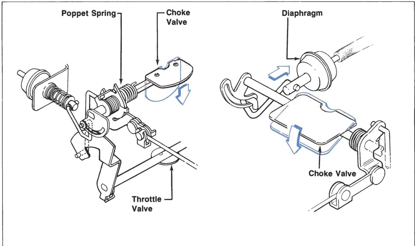
As soon as the engine starts, the air/fuel mixture must be leaned or the engine can stall (flood due to an over-rich mixture).
