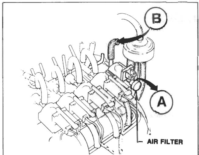
3. Disconnect the connector from the solenoid valve and connect the battery power to terminals on the valve.
