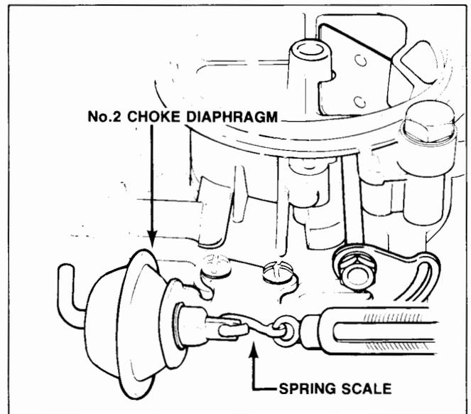
4. Reconnect the no.2 choke diaphragm connecting rod. Pull the choke lever link out fully and hold its position.
