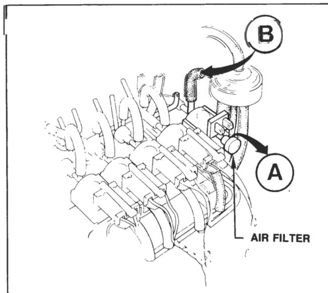
3. Disconnect the connector from the solenoid valve and connect the battery power to terminals on the valve.
