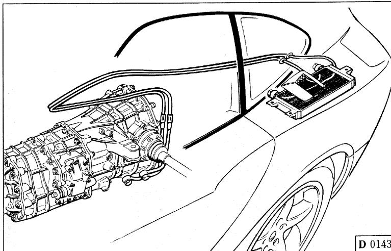
With plugs **A** and **B** screwed in, start the engine and allow the gearbox oil to reach a temperature of 185 + 194°F (85 + 90°C) in order to check if the densimetric valve has opened allowing oil to enter the oil cooling circuit.
