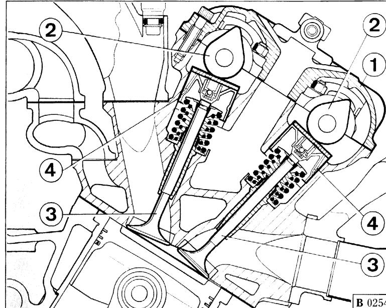
Valve timing features 4 head shafts (2 each cylinder bank) and 4 valves - two intake and two exhaust ones - each cylinder, driven by hydraulic tappets, having an automatic clearance recovery, thus keeping the same operating tolerance.
