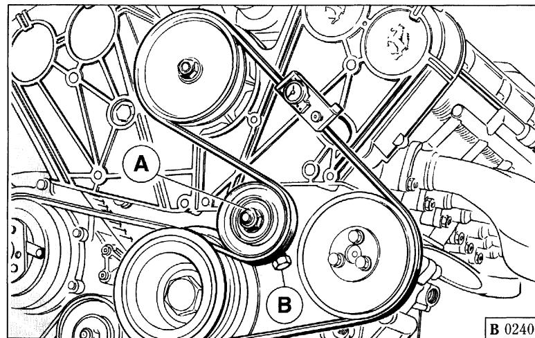
To adjust the belt tension, loosen the nut **A** (Fig. 9) locking the tensioner support, screw or unscrew the adjustment screw **B**, to reach the required tension, then lock again the nut **A**.
