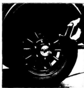
Figure 21a. Jack up the wheel until the tire clears the ground. Remove the dust cap and clamping nut from the valve stem. Remove the six rim clamps, unscrewing them with the brace wrench supplied in the tool kit.
