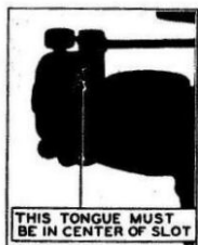
Figure 37. Before adjusting the carburetor, make sure that the enriching control rod is properly adjusted.
