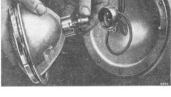
Fig. 38. Headlamp unit with adaptor removed.
