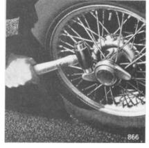
Fig. i8. Removing L.H. front hub cap.
