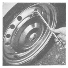
Fig. 17. Removing nave plate.
